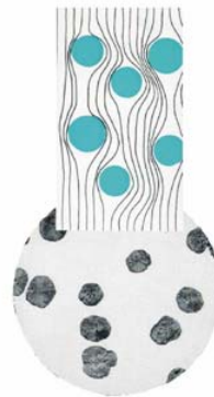
Duktilguss (Nodularguss, Sphäroguss) Graphit in Kugelform
